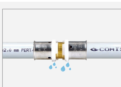
Unpressed fitting tested between 1 and 4.5 bar - not sealed
