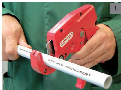
Cutting of pipe
