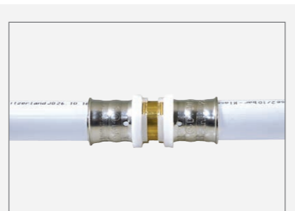
Pressed fitting tested at between 1 and 4.5 bar - sealed
